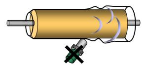
(2) Be sure to advance heat supply from one-end. In case of shrinkage from both ends, no air-pass is provided at the center, which may cause crease.
