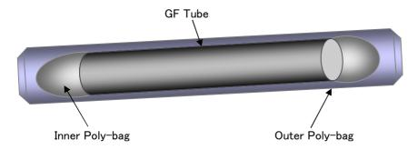
\* When carrying Tube or when applying Tube onto Roller, hang up Tube at Outer Poly-bag, not to push up Tube from bottom, in order to prevent Crease.
