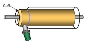
(4) Successively rotate Roller at constant speed, and proceed Blow Exit slowly while checking the boarder between shrunk and unshrunk area.
