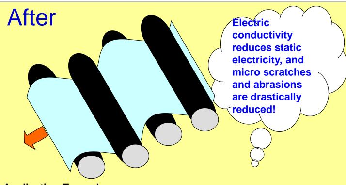
Application Examples: Manufacturing process and slitting process for film/ sheet
